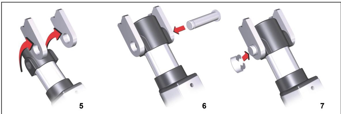
Figure 15 Steps for installing the stroke pipe (example)
