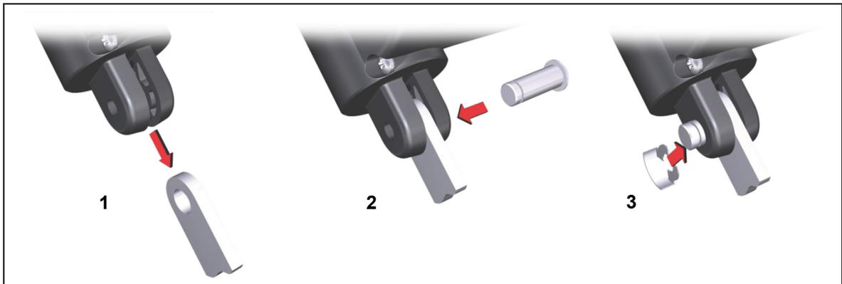
Figure 14 Steps for installing the gear clevis (example)
