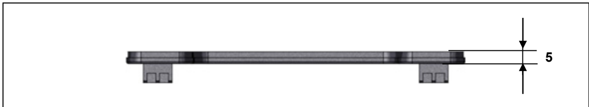
Figure 6 Dimensions of the CU165, side view (in mm)
